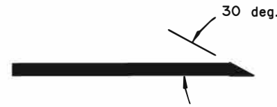
FIGURE 4 Safety Edge Detail
