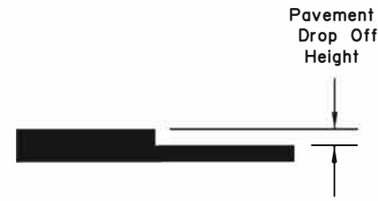
FIGURE 3 Pavement Drop-off Detail
