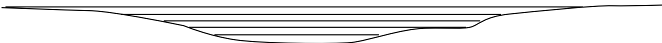
Figure 7.1. Deep repairs should be done in layers or “lifts” of no thicker than 8 inches and no less than twice the size of the largest aggregate.
