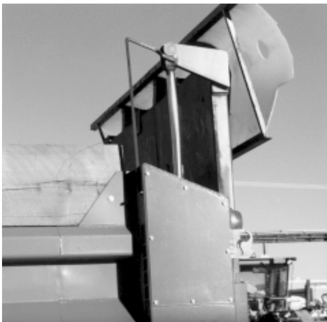
Figure 7.13. hydraulic, vertical action dump gate
