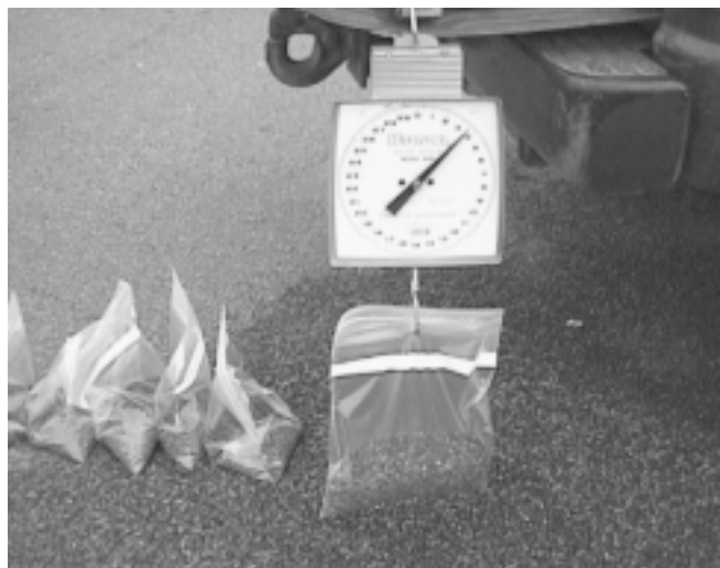
Figure 7.5. The contents of each bag are weighed and recorded.
