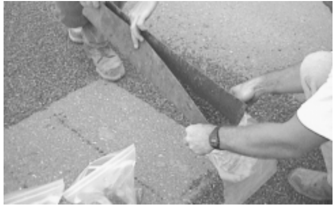
Figure 7.4. The aggregate on each mat is emptied into plastic bags.
