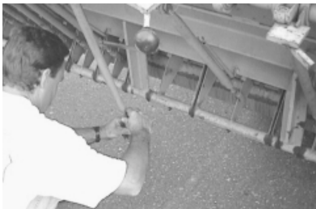
Figure 7.6. Adjusting a spreader gate opening.
