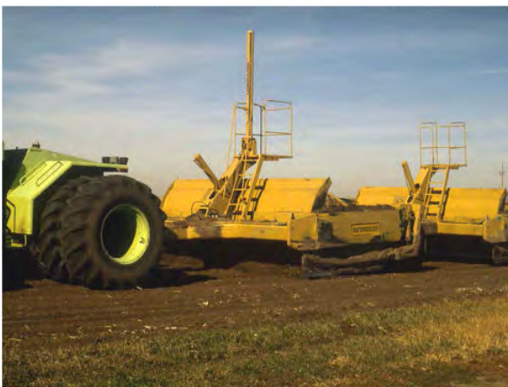
Figure 10.3. (a) Land grading and (b) planing in preparation for surface irrigation.
