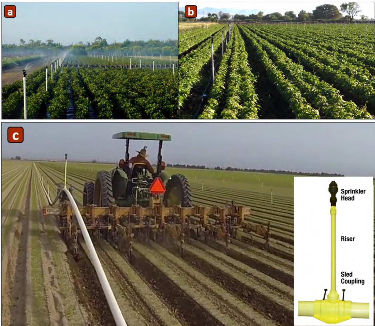
Figure 12.13. Examples of portable solid-set systems (photos a and b are courtesy of Hunter Industries; photo c is courtesy of Westlake Pipe & Fittings).
