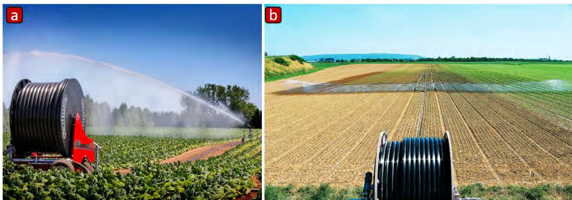
Figure 12.17. Hard-hose traveler diagram with photo of a traveler with a gun (photo a is courtesy of Cadman Power Equipment) and with large boom (photo b is courtesy of Bauer Group).
