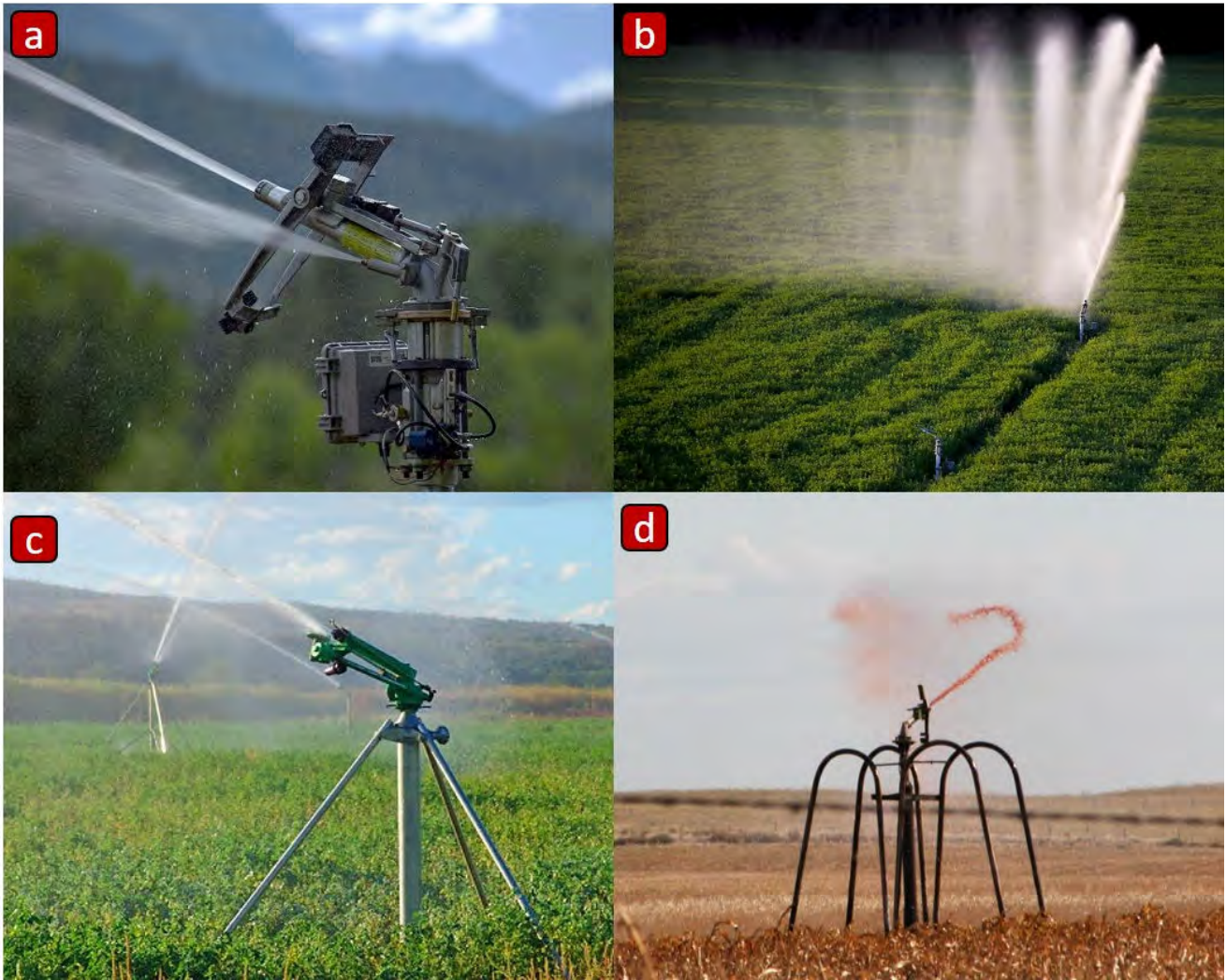
Figure 12.14. Illustration of gun sprinklers (photos a and b are courtesy of Nelson; photo c is courtesy of Wade Rain, Inc.).
