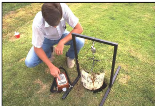
Small Weighing Lysimeter for Turf Grass Measurements
