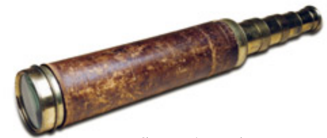
Shipmaster’s-type telescope with collapsible brass and wood-and-leather sections, made by William Cary, London, ca. 1802, owned by Meriwether Lewis.
