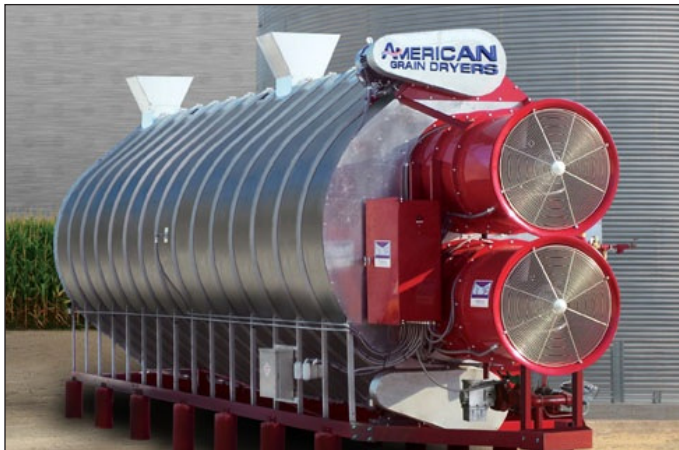
Figure 19: Stationary cross-flow batch dryer. Source: K. Hellevang
