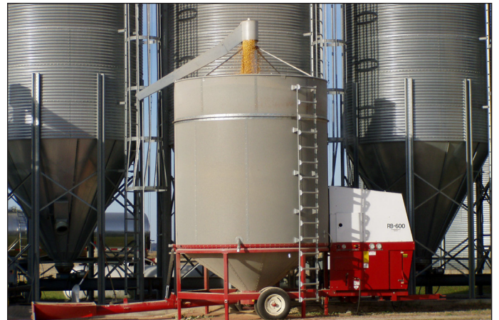
Figure 20: Recirculating Batch Dryer. Source: Scott Sanford
