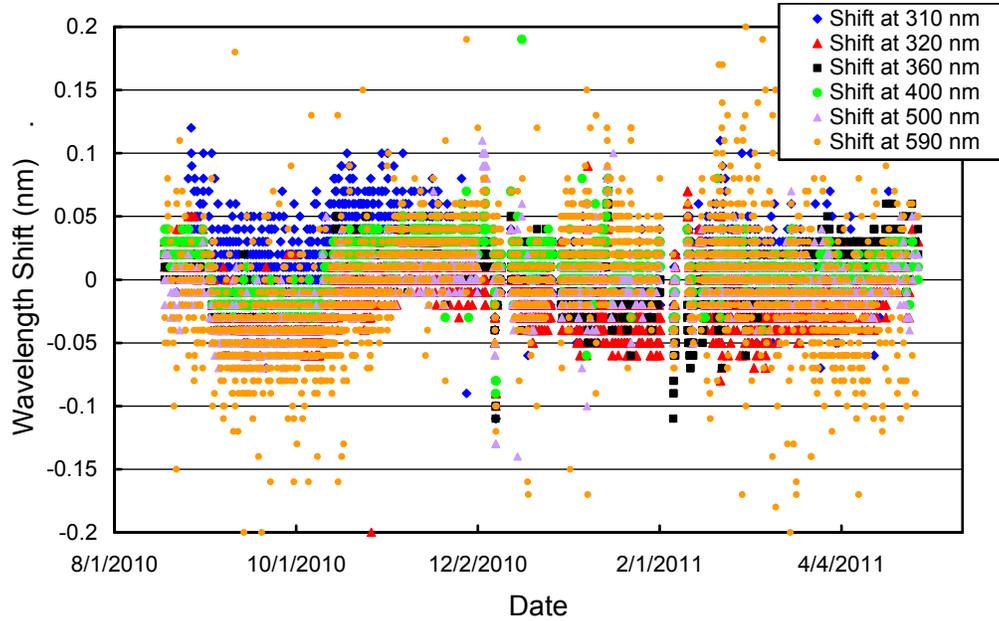
**Figure 5.1.6.** Check of the wavelength accuracy of final *Version 0* data at six wavelengths by means of Fraunhofer-line correlation. The plot is based on data measured at the top of the hour.
