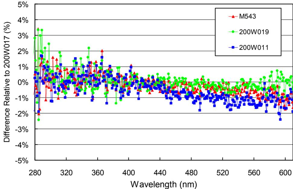
**Figure 5.1.1.** Comparison of McMurdo lamps M-543, 200W019 and 200W011 with the BSI traveling standard 200W017 on 02/02/11. The calibration of lamp 200W011 was established in 2008 while lamps M543 and 200W019 were calibrated against a weighted average of lamps 200W011 and 200W017.
