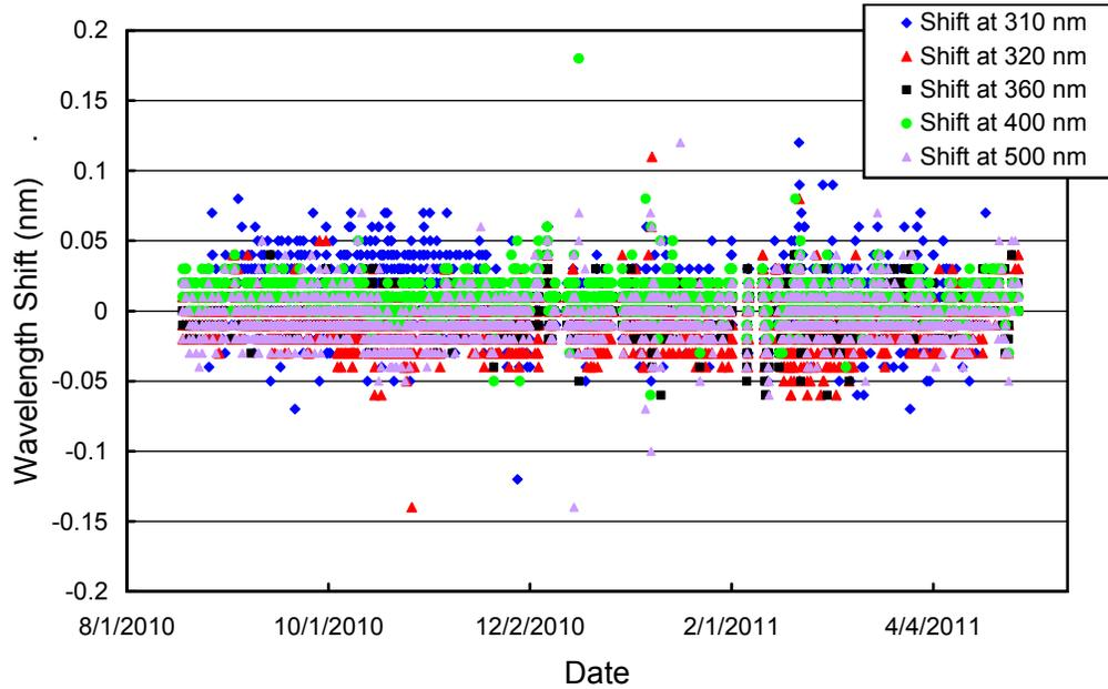
**Figure 5.1.2.** Check of the wavelength accuracy of final *Version 2* data by means of Fraunhofer-line correlation. The plot is based on data measured at the top of the hour.
