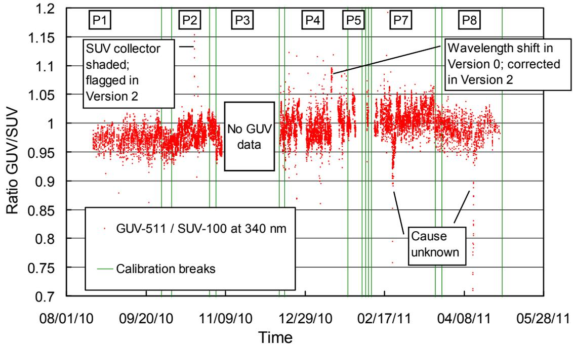
**Figure 5.1.2.** Ratio of GUV-511 measurements of its 340 nm channel with final SUV-100 measurements that were weighted with the spectral response function of this channel.
