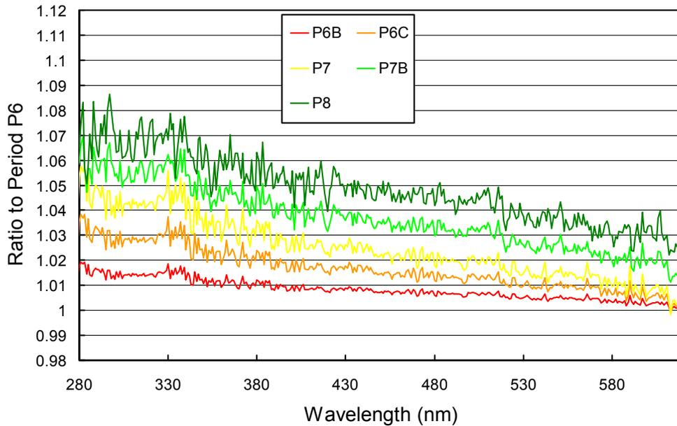
**Figure 5.1.4** Ratios of irradiance assigned to the internal reference lamp during periods P6B – P8, relative to Period P6.
