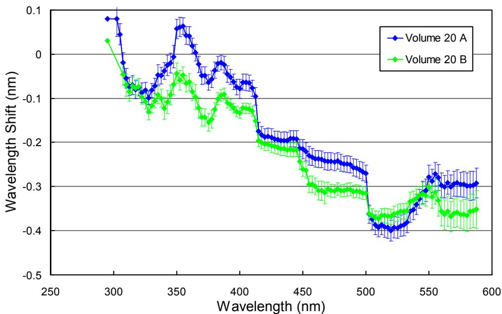
**Figure 5.1.5.** Monochromator non-linearity correction functions. Error bars indicate the  $1\sigma$ -variation. Period A (Period B) was applied to solar data recorded before (after) the February 2011 site visit. Instrument maintenance during this visit changed the correction function slightly.
