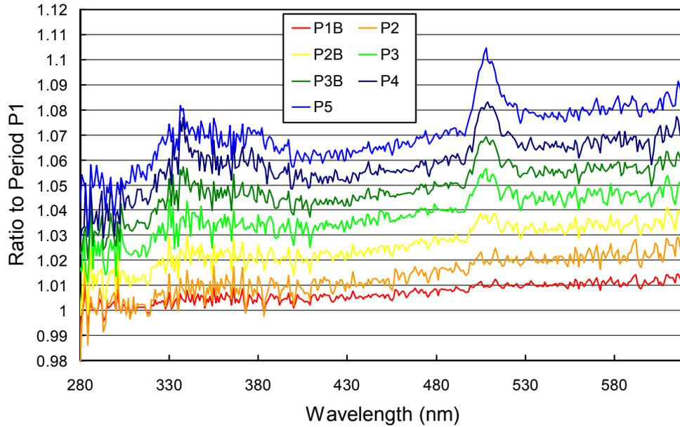
**Figure 5.1.3** Ratios of irradiance assigned to the internal reference lamp during periods P1B – P5, relative to Period P1. Changes from period to period are typically smaller than 2%.
