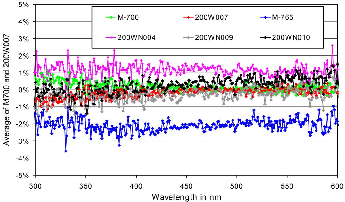
**Figure 2.** Comparison the calibration of on-site standards M700, 200W007, and M765, 200WN009, and 200W010, and the traveling standard 200WN004. The five on-site standards were measured on 3/28/15 while the traveling standards was measured on 3/29/15.
