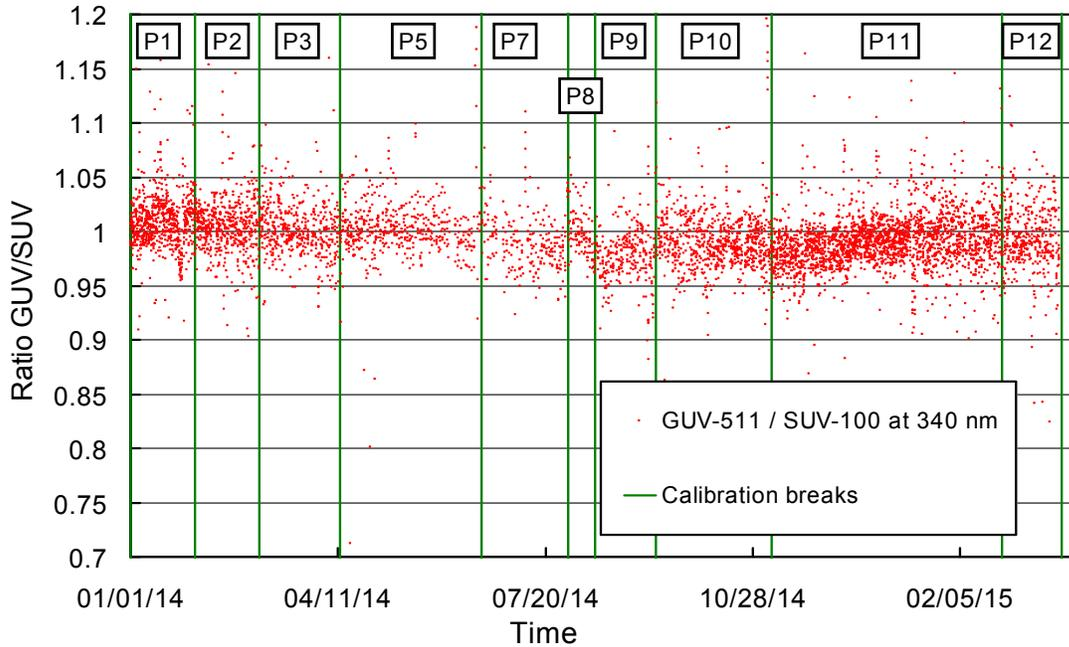
**Figure 5.** Ratio of GUV-511 measurements at 340 nm with final SUV-100 measurements. The latter were weighted with the spectral response function of the GUV-511 340 nm channel. Outliers with ratios larger than one are typically caused by measurements where the SUV-100 collector was covered by snow. Associated data have been flagged in the SUV-100 Version 2 data edition.
