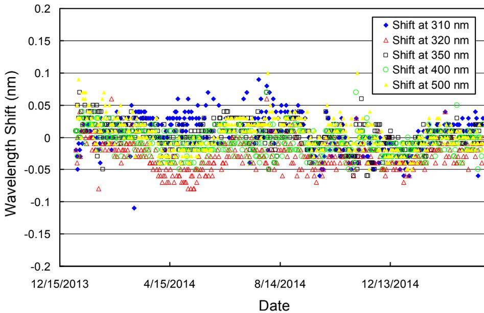
Figure 7. Wavelength accuracy check of the final data at five wavelengths by means of Fraunhofer-line correlation. Noontime measurements from every day of the year have been evaluated.
