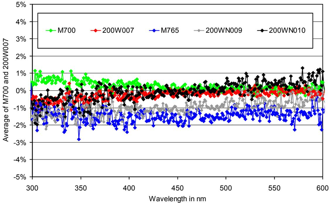
**Figure 1.** Comparison of the calibration of on-site standards M700, 200W007, M765, 200WN009, and 200WN010 on 3/21/2014. Data are reference to the average of the measurements of lamps M700 and 200W007.
