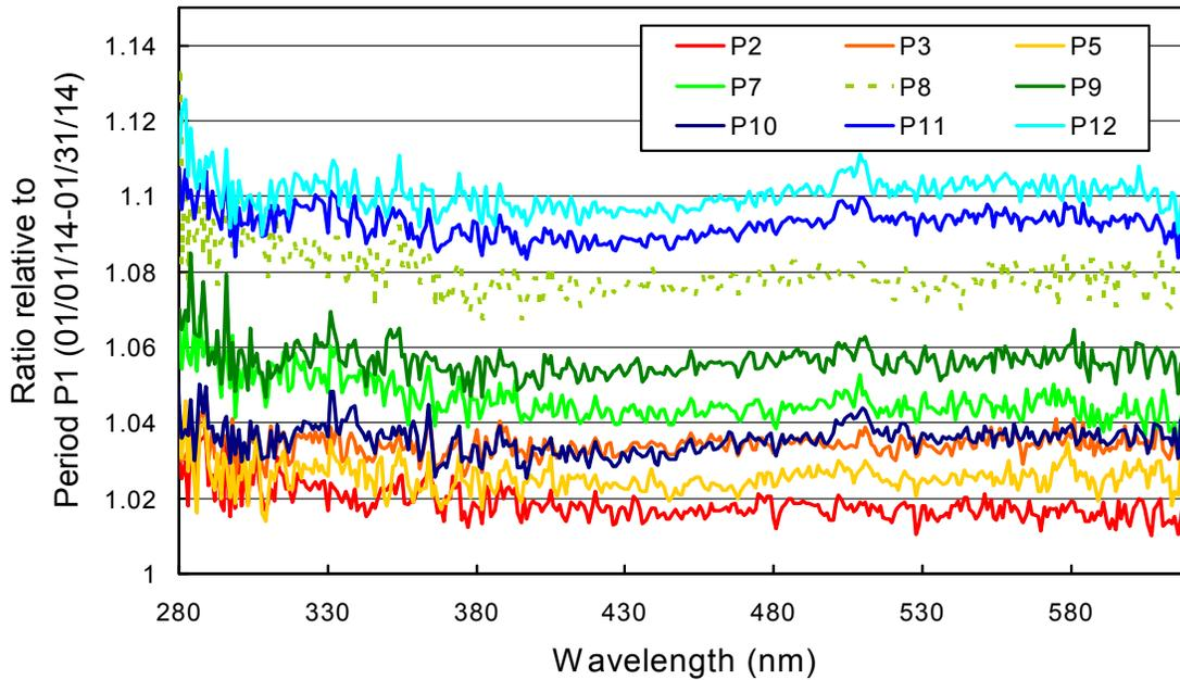
**Figure 4.** Ratios of spectral irradiance assigned to the internal reference lamp for periods P2 – P12 relative to Period P1.
