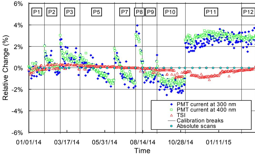
**Figure 3.** Time-series of PMT current at 300 and 400 nm, and TSI signal. All data were extracted from measurements of the internal irradiance standard and are normalized to their average. Calibration break points (Table 1) and times of absolute scans are also indicated.
