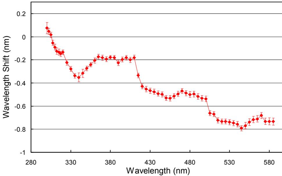
Figure 6. Monochromator mapping function.
