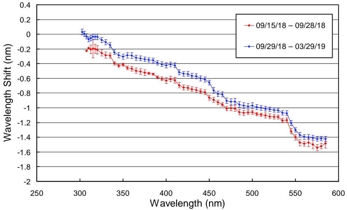
**Figure 3.5.** Monochromator non-linearity correction functions.
