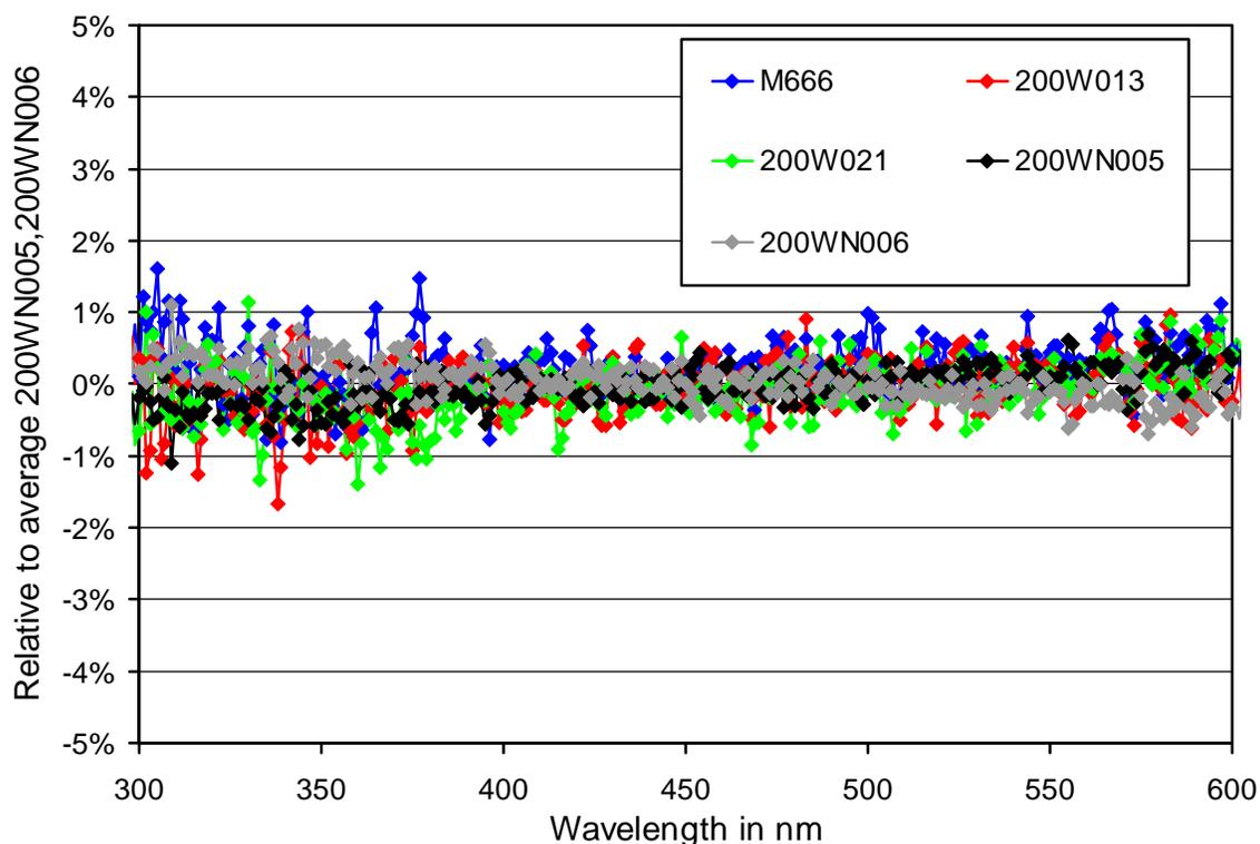
**Figure 3.1.** Comparison of South Pole lamps M-666, 200W021, 200W013, 200WN005 and 200WN006 on 11 and 12 September 2018.
