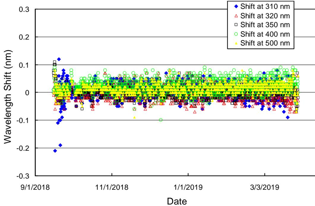
**Figure 3.7.** Wavelength accuracy check of *Version 2* data at five wavelengths by means of Fraunhofer-line correlation.
