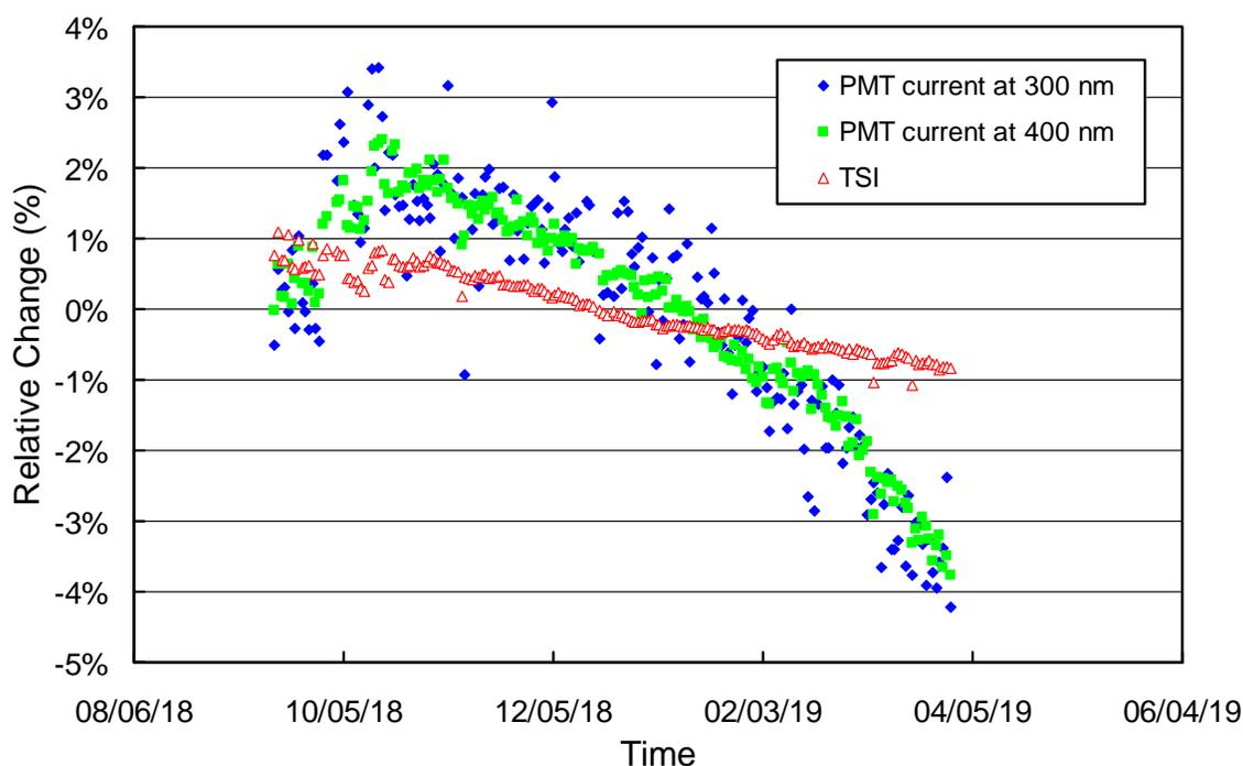
**Figure 3.2.** Time-series of PMT current at 300 and 400 nm, plus the TSI signal, derived from daily measurements of the SUV-100's internal irradiance standard. Data are normalized to the average of the whole period.
