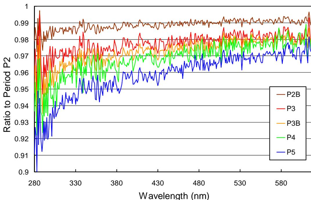
**Figure 3.4.** Ratios of spectral irradiance assigned to the internal lamp relative to the spectral irradiance of Period P2.
