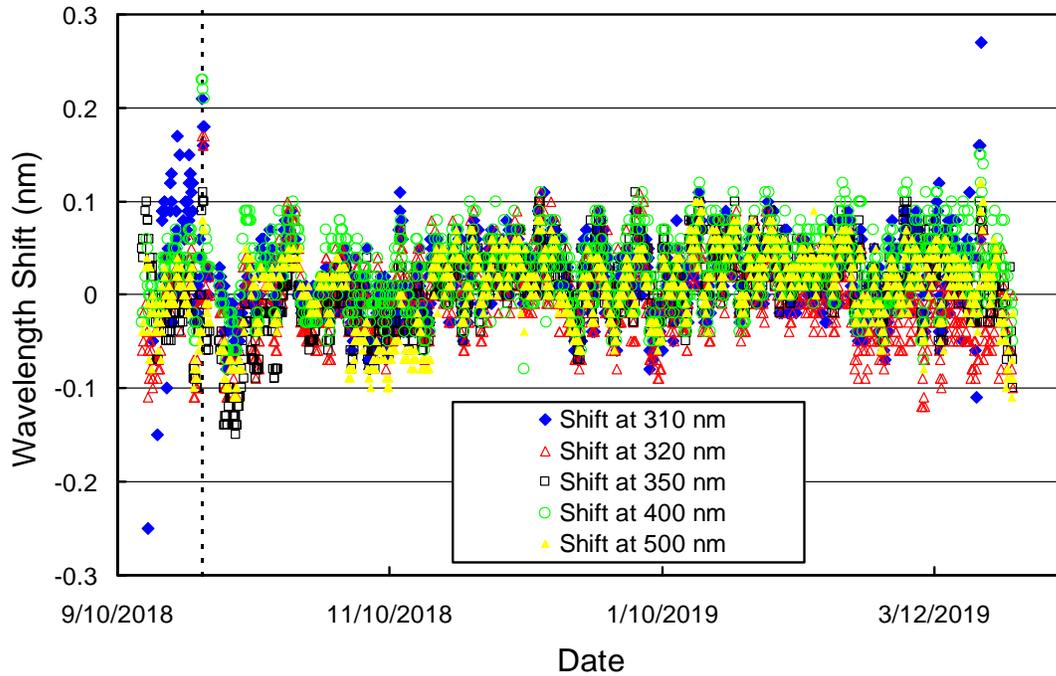
**Figure 3.6.** Wavelength accuracy check of *Version 0* data at five wavelengths by means of Fraunhofer-line correlation. The vertical broken line indicates the time when the collector was cleaned.
