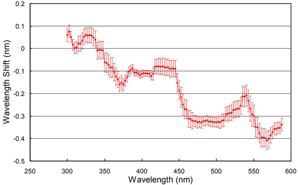
**Figure 5.** Monochromator non-linearity correction function for the Volume 31 period. Error bars indicate the  $1\sigma$ -variation.
