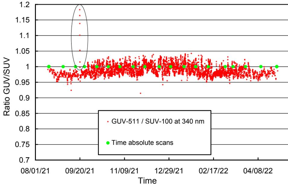
**Figure 4.** Ratio of GUV-511 (340 nm channel) and SUV-100 measurements. The times when “absolute” calibration scans of the SUV-100 were performed are indicated by green symbols. The ellipse marks outliers which were likely caused by snow covering the collector of the SUV-100 but not the GUV-511.
