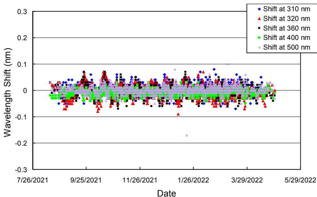
**Figure 7.** Check of the wavelength accuracy of Version 2 data at six wavelengths by means of Fraunhofer-line correlation.
