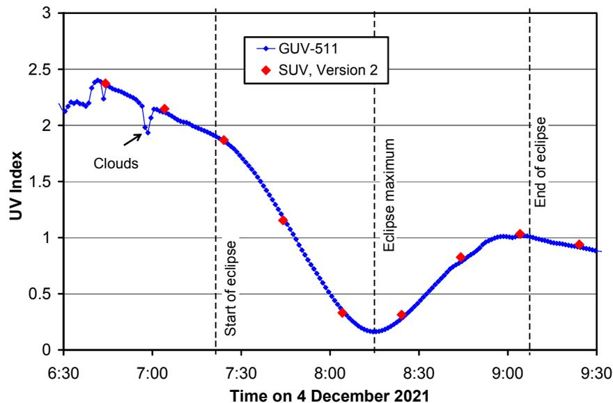
**Figure 1.** UV Index at the McMurdo during the solar eclipse of 12/4/21. Measurements by the SUV-100 spectroradiometer (Version 2 data) and GUV-511 radiometer are in good agreement. During the eclipse maximum, the UV Index is about 13% of the value expected from the unobstructed Sun. Measurements were slightly affected by clouds.
