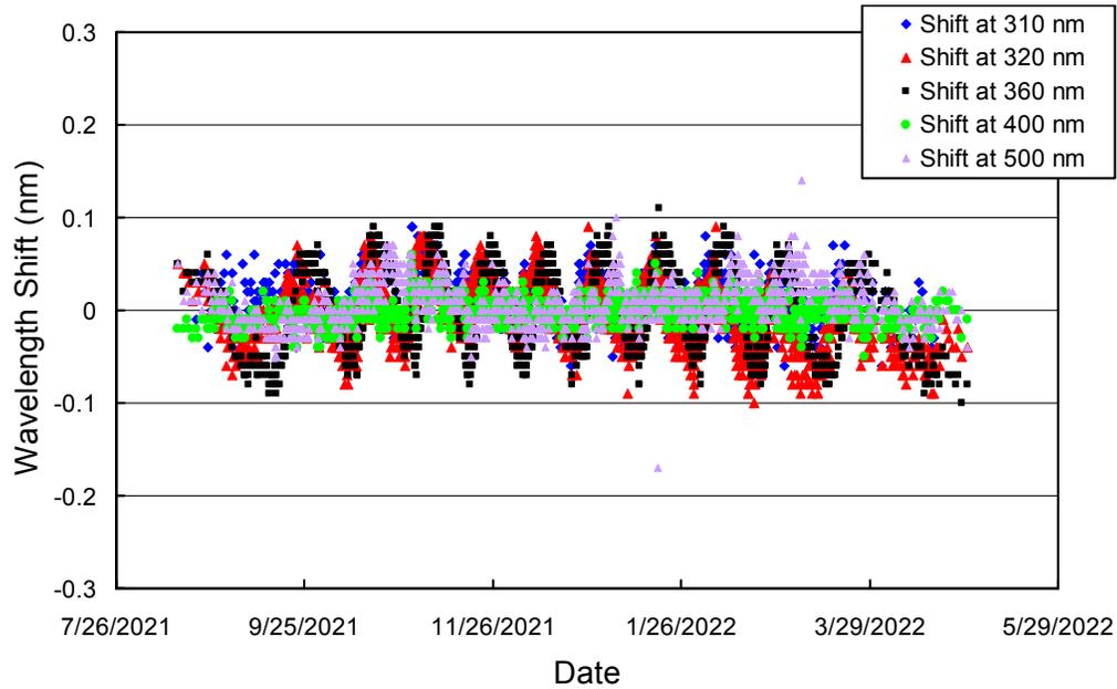
**Figure 6.** Check of the wavelength accuracy of Version 0 data at six wavelengths by means of Fraunhofer-line correlation. The plot is based on measurements that are three hours apart.
