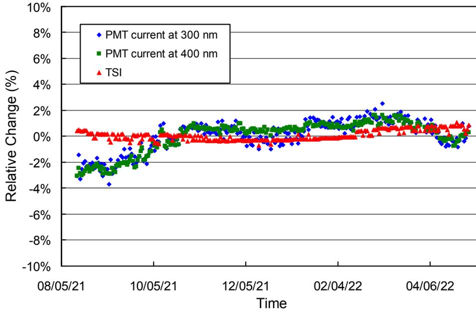
**Figure 3.** Measurements of the SUV-100’s TSI sensor and PMT currents at 300 and 400 nm. Data are shown as relative change and normalized to the average of the entire period.
