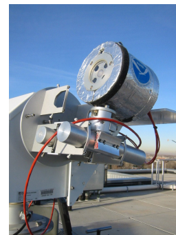
Figure 2. A 4-channel SP02 Sun Photometer was modified for monitoring AOD at BRW during winter 2012/2013.
