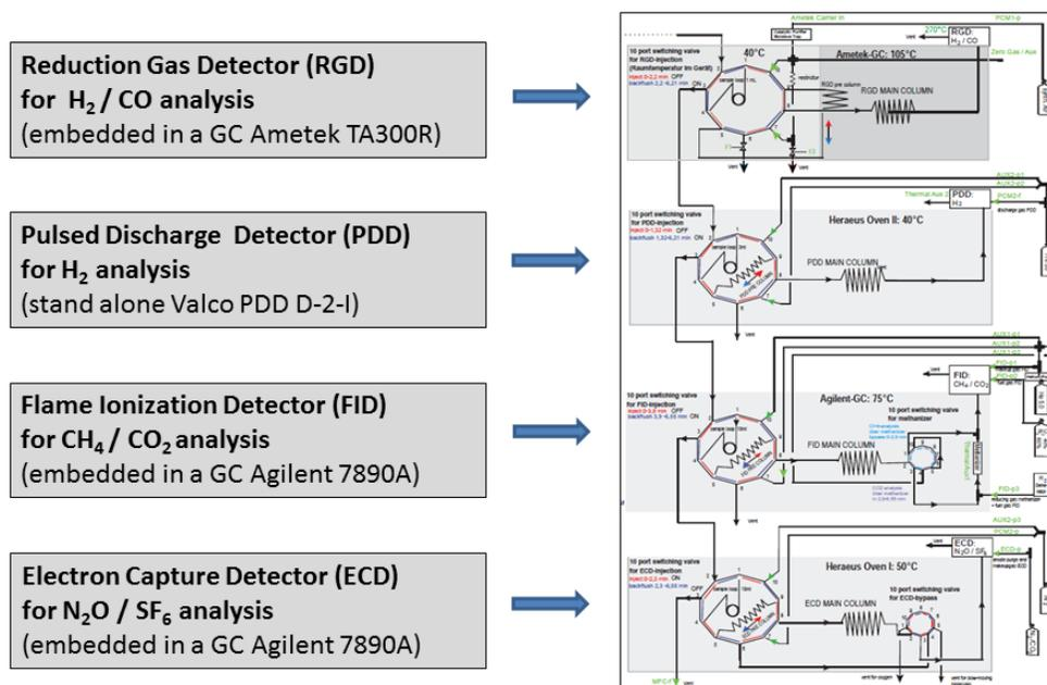
**Figure 1.** Setup and parallel operation of the GC trace gas analysis line.
