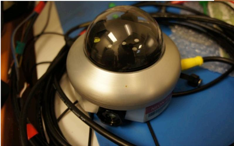
Dynamax SPN1: Direct & Diffuse Pyranometer (400-2700 nm)
