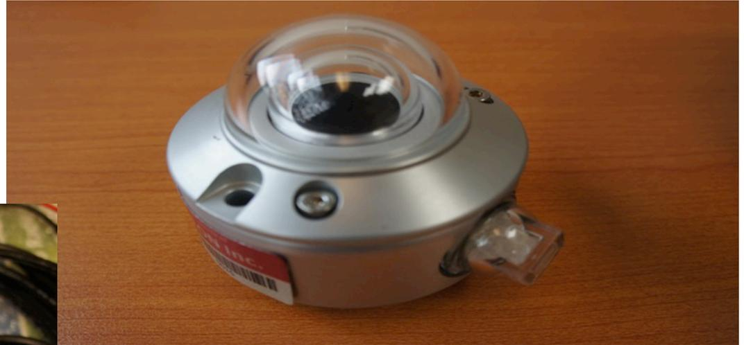
Kipp & Zonen CMP22: Primary Pyranometer ISO Standard (200 to 3600 nm)
