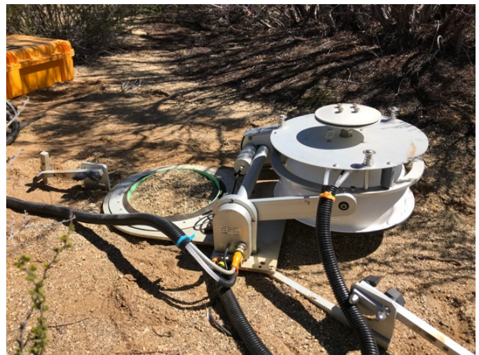
Figure 2. LI-8100 long-term chamber placed 150 cm from redshank trunk at Sky Oaks Field Station.
