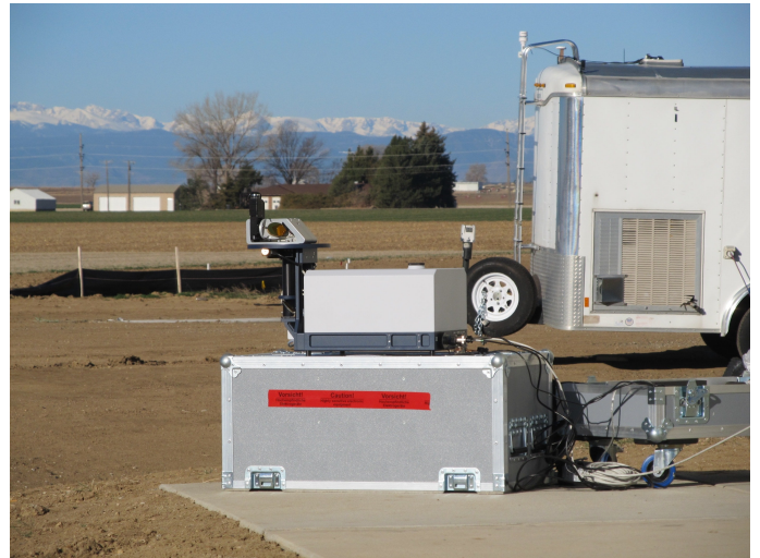
Figure 2. One of the COCCON instruments measuring \text{CH}_4 at the main measurement site inside the Denver-Julesburg Basin. CU SOF, deployed in the trailer, measured the NG and agricultural tracers.
