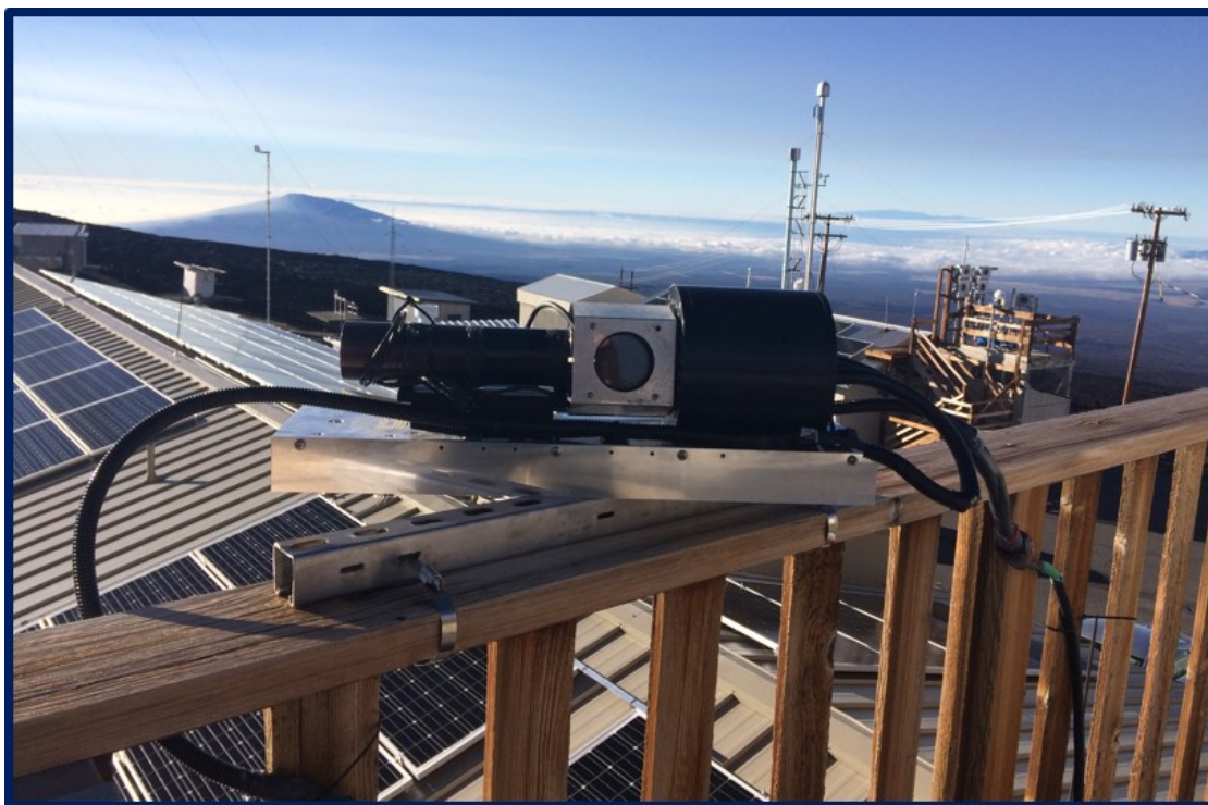
Figure 1. A view over the MLO MAX-DOAS telescope (pictured here without its protective cover) in the primary scanning direction. Light is collected through viewing port (face on here) and sent to two spectrometers for analysis via optical fibers. By rotating in the vertical plane, spectra can be collected along lines of sight pointing below, at, and above instrument altitude. The instrument has collected data on a variety of tropospheric and stratospheric trace gases since February 2017.
