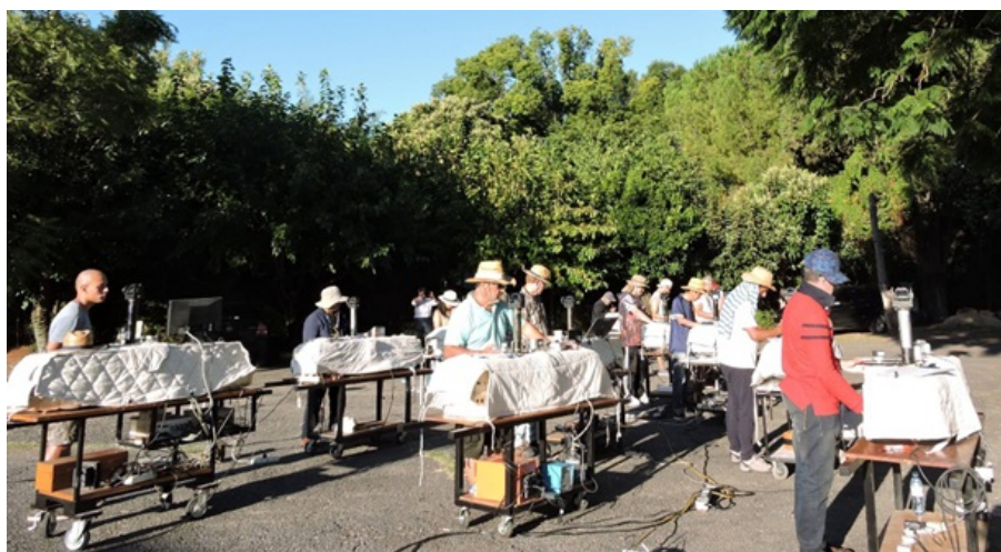
Figure 2. The final intercomparison of all the participating Dobson instruments and the U.S.A. world Secondary Dobson (D065) on March 18, 2019.
