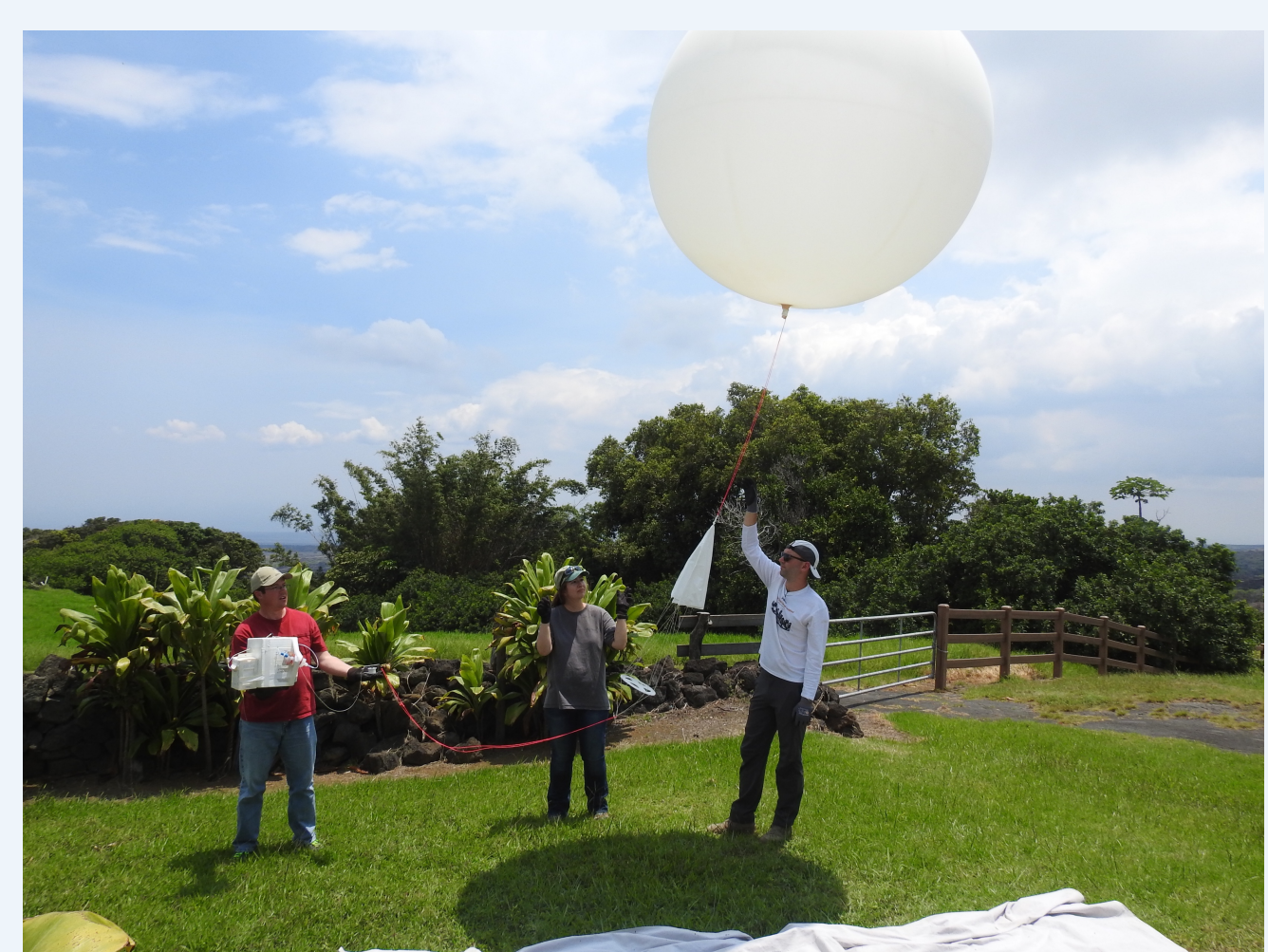
Figure 3. Launch of single-pump SO 2 sonde at Kahuku Ranch located at the "June launches" site on Figure 2.
