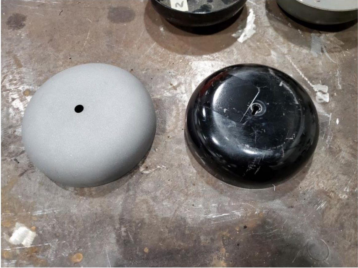
Figure 6. Alarm bells shown before and after finishing. Left bell (finished, right bell (unfinished).
