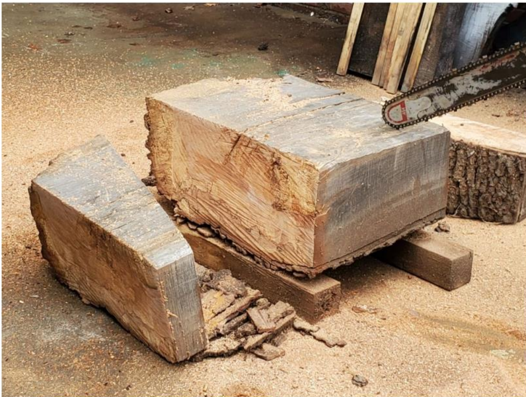
Figure 1. Wood being cut down to workable sizes with a chainsaw.
