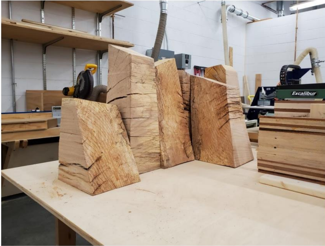
Figure 2. Select wood blocks after shaping with various power tools. Shaping took place to maximize the exposure of naturally occurring slices which help the wood to resonate.
