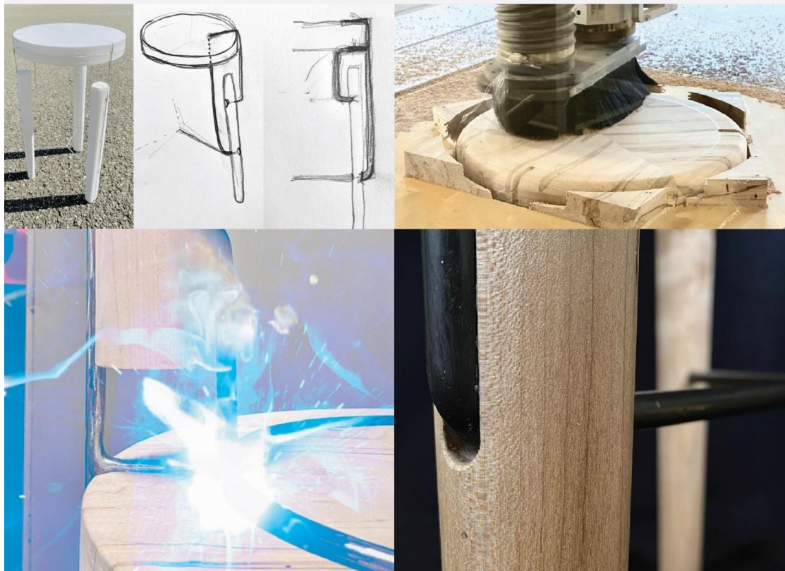
Image 4: exploded axon, physical model, sketches, CNC milling of seat deck, welding of structural system, and detail image of joinery for Selah [she-luh] stool design (from left to right, descending order)
