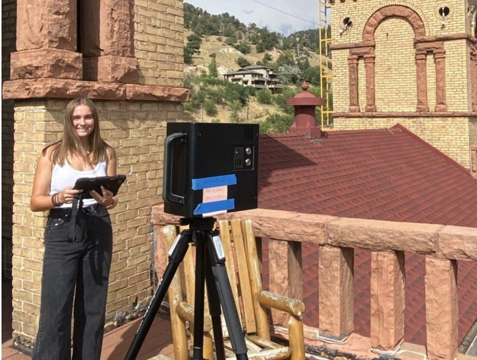
The AVL research intern scans a 3D historic building using Matterport technology.
