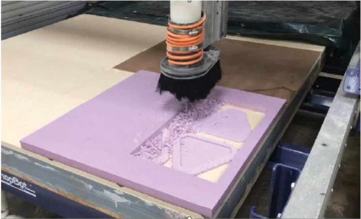
FIGURE. 03- Fabrication using CNC machine and foam
