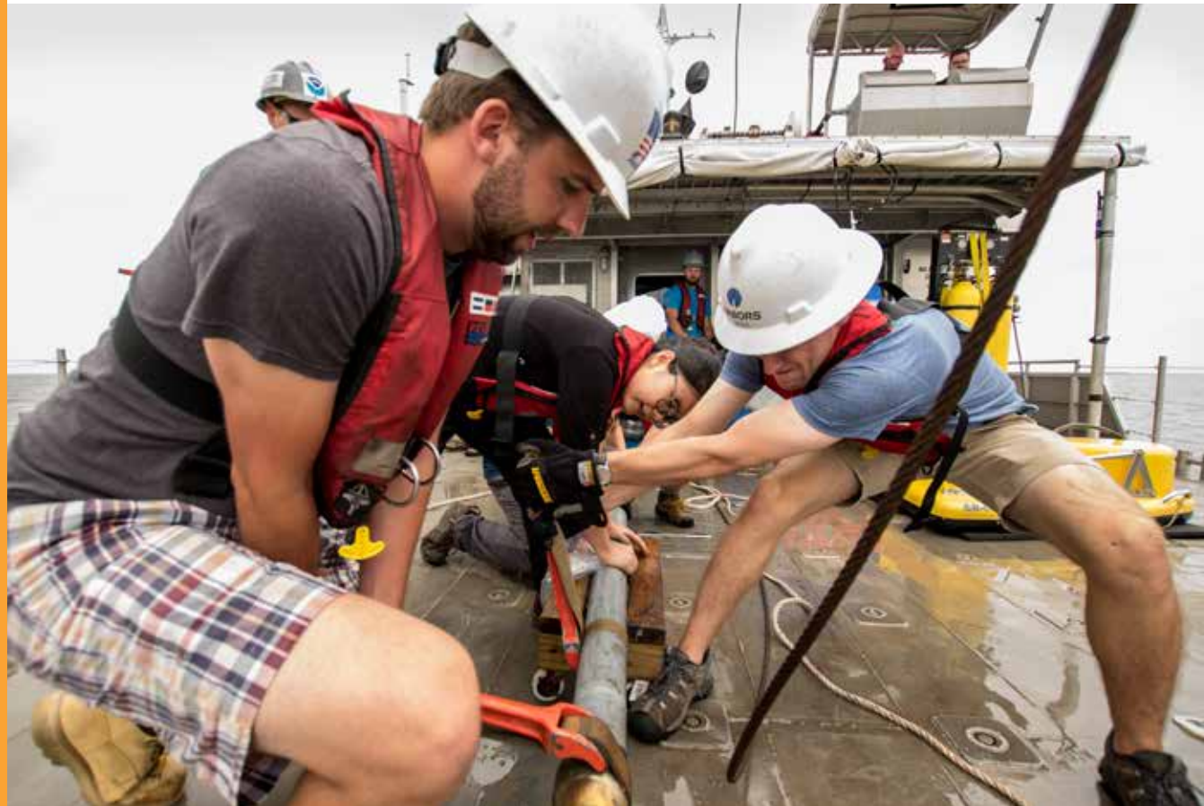
STUDENTS READY A PISTON CORER FOR OFFSHORE SEDIMENT SAMPLING NEAR GALVESTON. CREDIT: RODRIGO FERNANDEZ
