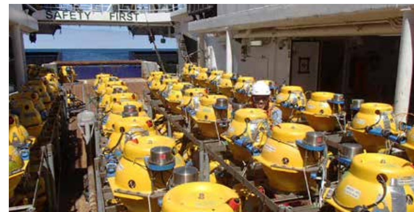
OCEAN BOTTOM SEISMOMETERS AWAIT DEPLOYMENT ON THE DECK OF A RESEARCH VESSEL NEAR NORTHEAST NEW ZEALAND. THE INSTRUMENTS AID UTIG SCIENTISTS IN UNDERSTANDING EARTH'S CRUSTAL STRUCTURE. CREDIT: HARM VAN AVENDONK
