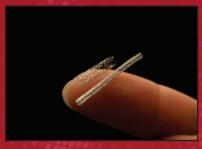
Whether the part is a dental post, or a full hip replacement, IMR can analyze these surfaces by ferroxyl swab testing. This is used to detect free iron on implants at very low levels.
