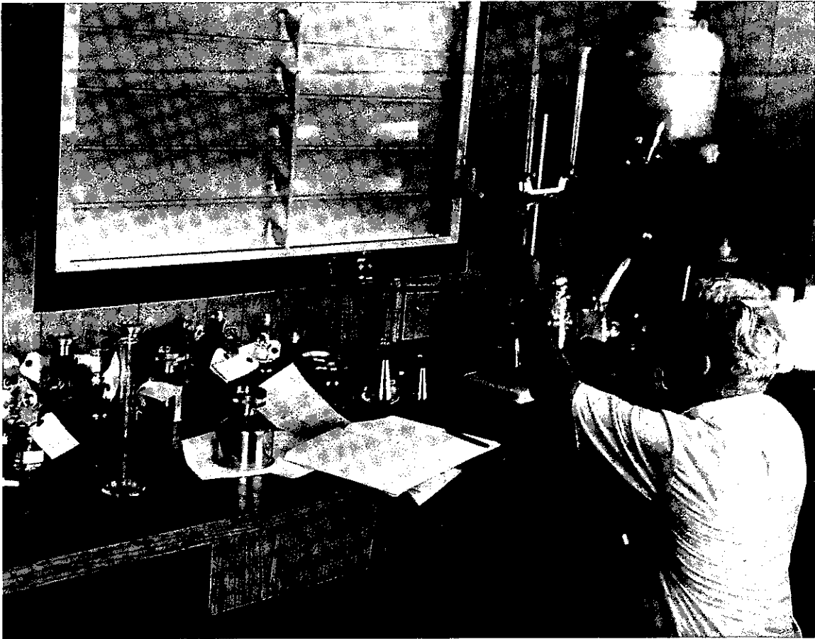
Figure 5. Oxygen titrations, coliform bacteria filtrations and reagent preparations were performed at the lake site, in the small mobile laboratory.
