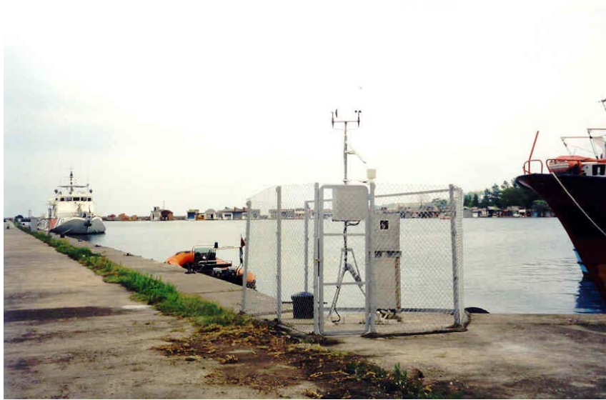
Figure-3.7: Trabzon digital and automatic tide gauge
