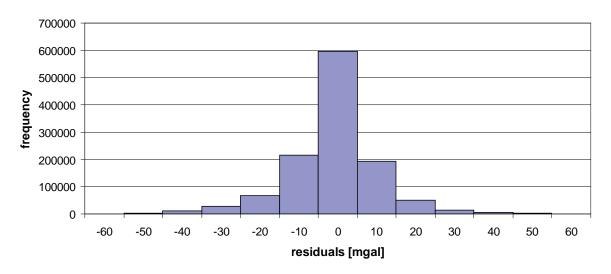
Fig. 10: Histogram of comparing the  $5' \times 5'$  African free-air gravity anomaly database AFRGDB\_V1.0 with real data. (After Abd-Elmotaal et al., 2014).
