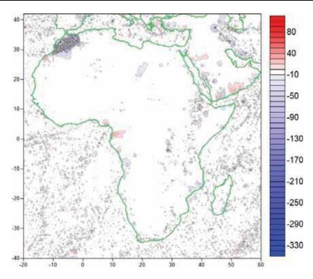
Fig. 9: Residuals at the data points between measured values and the  $5' \times 5'$  African free-air gravity anomaly database AFRGDB\_V1.0. Contour interval: 10mgal. (After Abd-Elmotaal et al., 2014).
