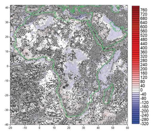
Fig. 8: The 5'  $\times$  5' African free-air gravity anomaly database AFRGDB\_V1.0. Contour interval: 20 mgal. (After Abd-Elmotaal et al., 2014).
