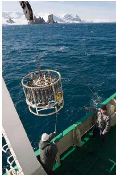
A Conductivity, Temperature and Depth (CTD) cast in Bransfield Strait, Antarctica (photo: V. Morozov).
