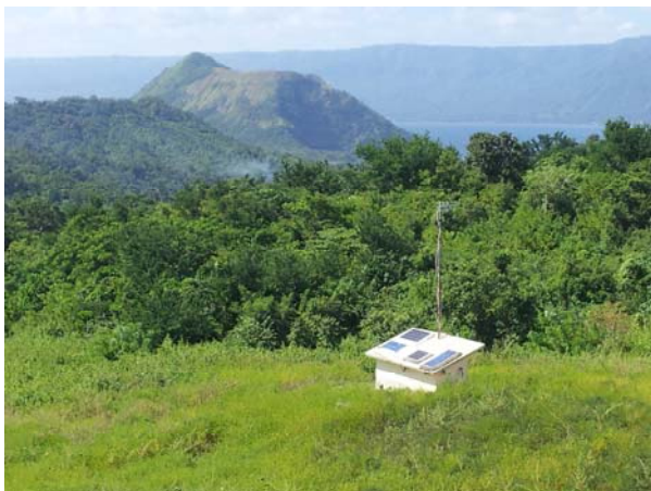
Telemeter multiparameter station on Taal volcano
