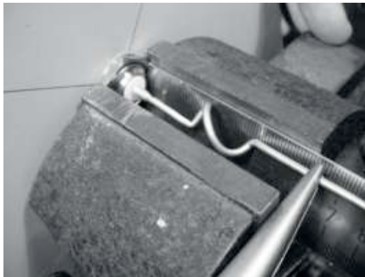
Figure 4.30: Stretching the coils. Be very gentle and try not to scrape the surface of the wire with the pliers.
