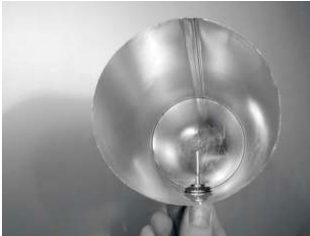
Figure 4.42: Your finished cantenna.
