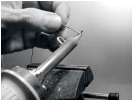
Figure 4.26: Add a little solder to the end of the wire to “tin” it prior to soldering.
