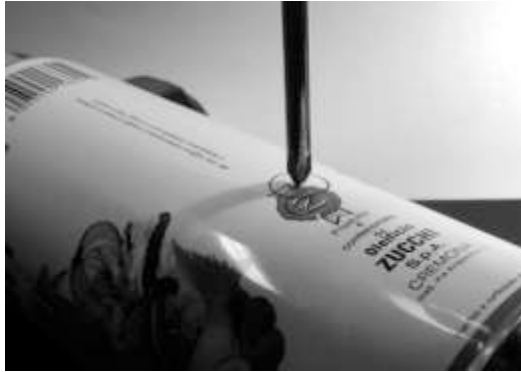
Figure 4.36: Mark the hole before drilling.
