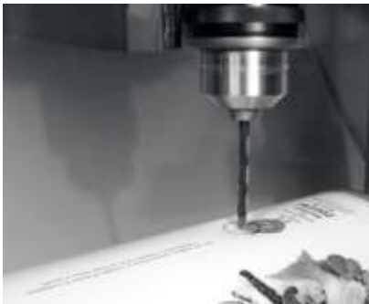
Figure 4.37: Carefully drill a pilot hole, then use a larger bit to finish the job.
