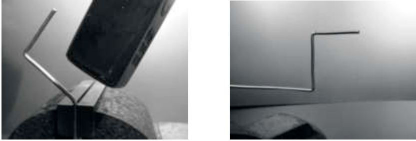
Figure 4.17: Bend the wire into a "Z" shape.
