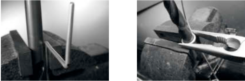
Figure 4.18: Bend the wire around the drill bit to make a coil.
