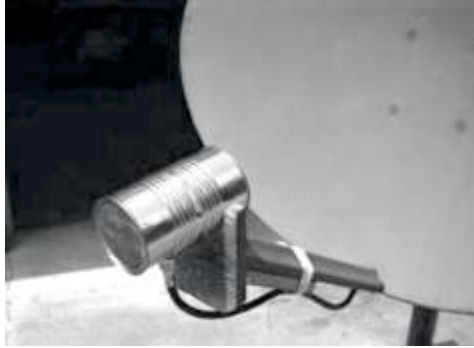
Figure 4.10: Feed horn made from a food can.
