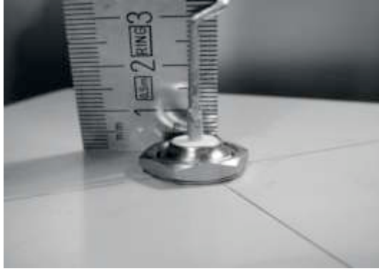
Figure 4.27: The first coil should start 3.0 cm from the surface of the plate.
