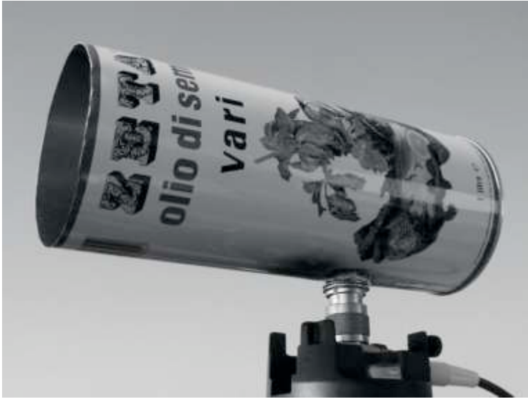
Figure 4.33: The finished antenna.
