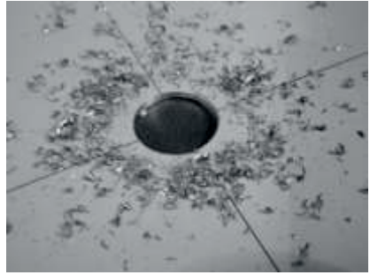
Figure 4.22: Drilling the hole in the metal plate.
