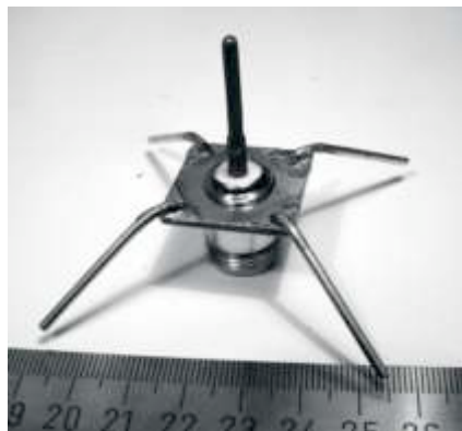
Figure 4.8: Quarter wavelength ground plane antenna.
