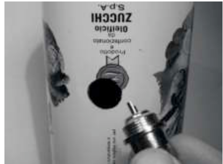
Figure 4.37: Carefully drill a pilot hole, then use a larger bit to finish the job.
