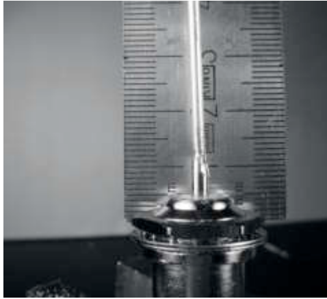
Figure 4.40: The length of the wire is critical.
