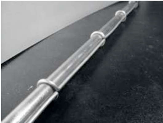
Figure 4.21: Inserting a pipe can help to straighten the wire.
