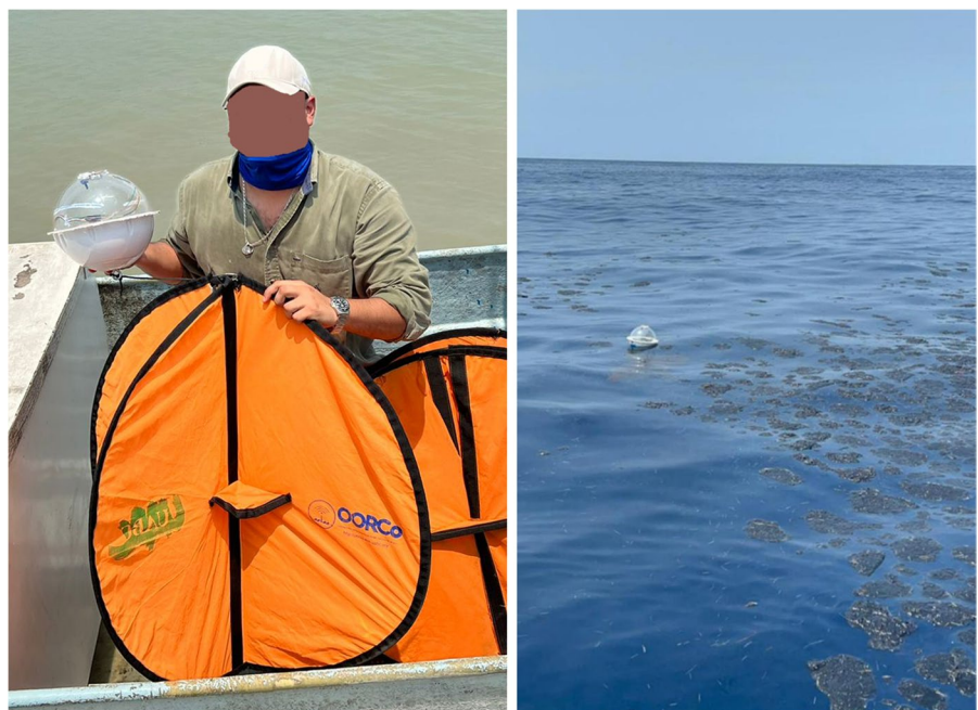
Fig. 3 On-site deployment of DORIS buoys in an area where an oil slick was detected by satellite. The image shows the oil tars on the sea's surface, inserted into an oil–water matrix that singularly reflects sunlight and is detected by optical sensors on satellites, as well as by SAR because the oil flattens the surface of the sea
