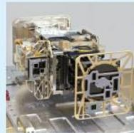
EXIS detects and monitors solar irradiance in the upper atmosphere. The X-Ray Sensor monitors solar flares that can disrupt communications and degrade navigational accuracy, affecting satellites, astronauts, high latitude airline passengers and power grid performance.
