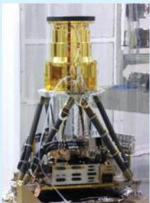
GLM will be the first-ever operational lightning mapper flown from geostationary orbit. GLM maps total lightning (in-cloud and cloud-to-ground) activity continuously day and night over the Americas and adjacent ocean regions. Research and testing has demonstrated GLM's potential for improvement in tornado warning lead time and false alarm rate reduction.
