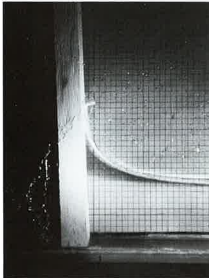
Fluid Mechanics. Researchers at the Massachusetts Institute of Technology, seeking to predict the seaworthiness of vessels and offshore structures in sudden storms, performed an experiment illustrated in this photograph. It shows the formation of a jet at the free surface of a liquid being accelerated by the impulsively moved plank on the left. The experiment was compared with computed time-sequence behavior of the free surface under similar conditions.
