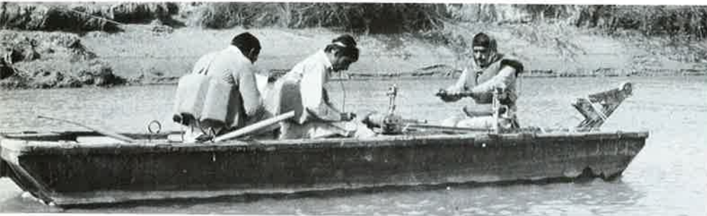
Field measurements of sediment transport. These measurements in Pakistan's Link Canals verify laboratory research results. They are part of a cooperative research project with Khalid Mahmood, at George Washington University, and researchers at the Water and Power Development Authority in Pakistan.
