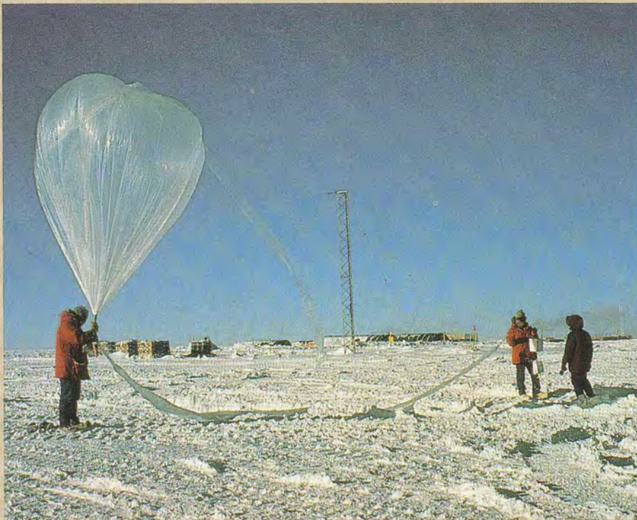
On the rise. Researchers at the South Pole launch a balloon carrying ozone-measuring instruments. Similar balloons have been used near the North Pole, where chlorine from CFC's also plays a key role in ozone depletion.
