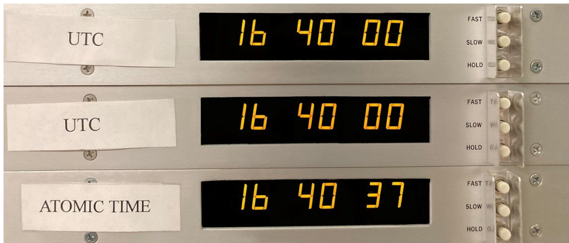
Fig. I.A.16. Photograph of three impulse clocks driven by the primary UTC(NIST) PPS; each time code advances by one second whenever a PPS is received. The clocks are not networked and receive no other time- or frequency reference. Impulse clocks labeled "atomic time" are never adjusted to account for leap seconds; "UTC" time codes are manually corrected for new leap second insertions by manual use of the "hold" interlock switch shown here. Though this is a very coarse validity test of UTC(NIST), disagreements between these impulse clocks can help diagnose certain failure modes in the PPS generation/distribution network to which several high-resolution tests are insensitive.
