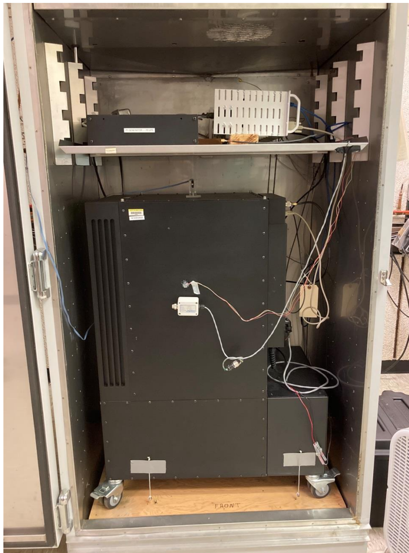
Fig. I.A.6. Hydrogen maser in an environmental control chamber with its door open. The shelf above the maser holds a redundant DC supply (left) for the distribution amplifier and monitoring rack (right).
