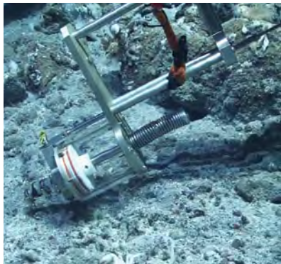
LEFT: QUEST 4000 taking “syringe” sample of microbial-rich sediment near hydrothermal vent at 2,390 m for natural products research program at Oregon State University, College of Pharmacy. The sample will be screened for compounds that could lead to new drug development.
