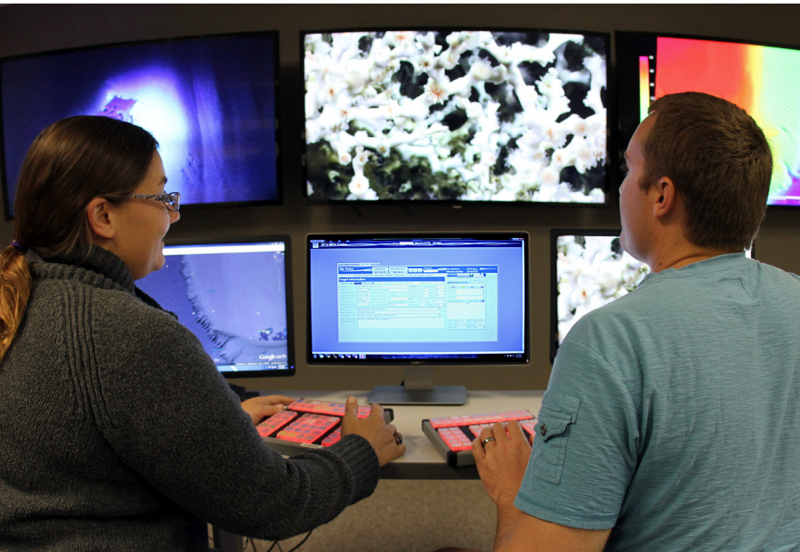
Scientists at Florida Atlantic University's Harbor Branch Campus have developed a programmable "hot keypad" system and database that was tested during the OER 2014 Exploration of the Gulf of Mexico. The system allows scientists to rapidly and accurately annotate observations with complete taxonomic information while observing the live video stream. Faculty there also developed structured curricula that use real-time datasets to provide students with real-world data analysis and annotation experience. Credit: B. Cousin, FAU Harbor Branch.
