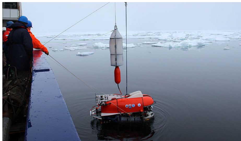
Nereid two-body system being deployed from the Polarstern during August 2014 sea trials. The mated-depressor and tow-body are lifted above the vehicle to facilitate a single point lift. Credit: C. German, WHOI.
