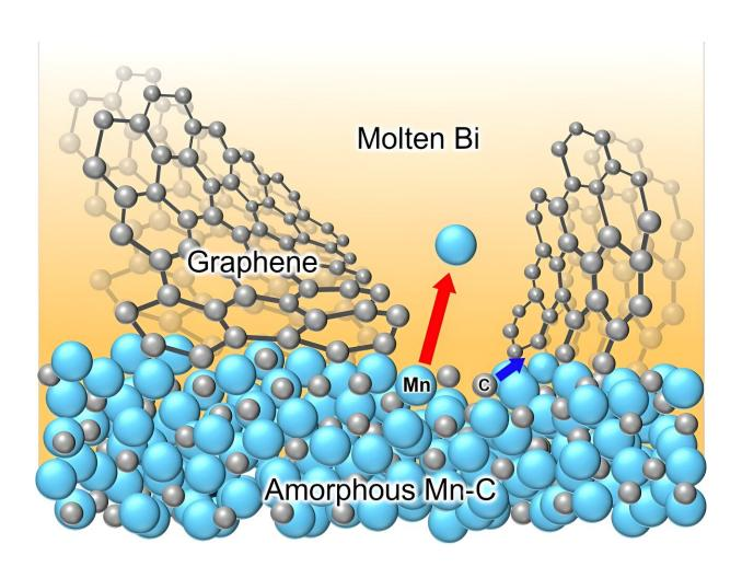
Schematic illustration for the formation NCG during liquid metal dealloying of amorphous manganese-carbon (Mn-C) alloy in a molten bismuth (Bi) to induce selective dissolution of manganese (Mn) atoms and self-organization of carbon (C) atoms into graphene layers. Credit: *Advanced Materials* (2024). DOI: 10.1002/adma.202311792
