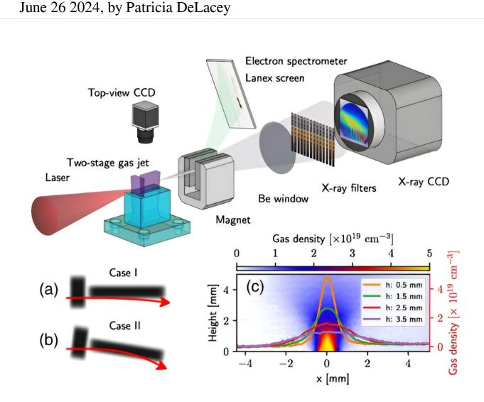
Experimental setup. A laser pulse was focused on a two-stage gas jet to produce electron and betatron x rays. (a) and (b) The schematic of the laser-target geometry in the two cases, respectively. The red arrows represent the laser trajectories. (c) Measured averaged transverse neutral gas density distribution at a backing pressure of 4.1 MPa and gas density profiles at different heights above the nozzle for the accelerator. Credit: *Physical Review Letters* (2024). DOI:
