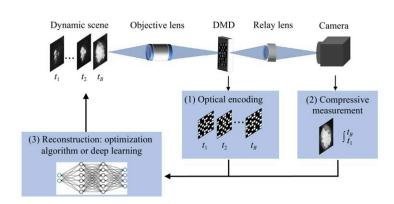
Principle of snapshot compressive imaging, which consists of optical encoding, compressive measurement, and reconstruction. Credit: *Light: Advanced Manufacturing* (2024). DOI: 10.37188/lam.2024.029
