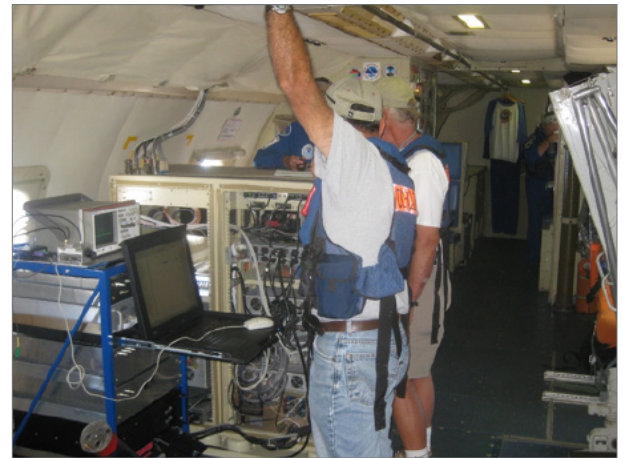
ESRL engineers checking out the W-band radar instrumentation during test flights on the NOAA P-3 near Tampa, FL. Credit: NOAA
