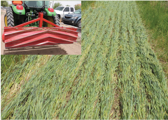
Figure 6. Terminating a winter cereal cover crop with a roller–crimper.
