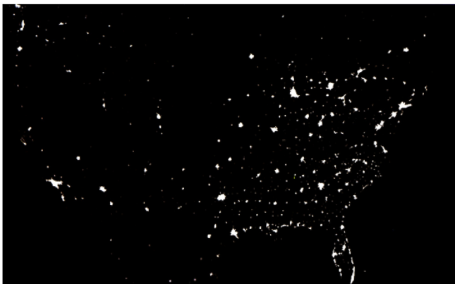
Fig. 8. NGDC's first map of DMSP nighttime lights, produced from 29 orbits and no cloud screening.
