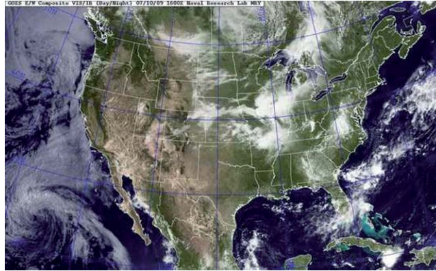
Fig. 2 GeoColor imagery from the NexSat website. The static color background is composed of images from NASA's blue marble (MODIS data) and current GOES visible and infrared data overlaid via dynamic transparency factors.
