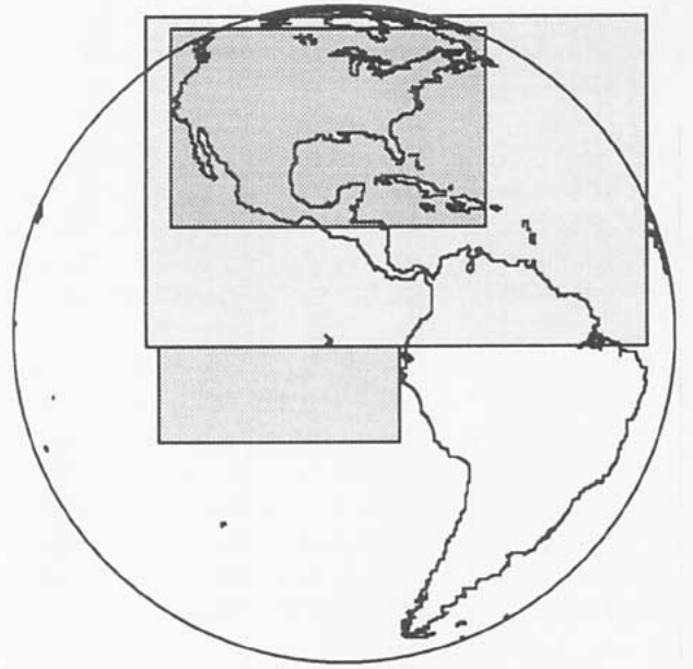
FIG. 5b. Coverage using the GOES-I imager in the warning mode. Half-hour sequence proceeds as follows: Northern Hemisphere frame (covering down to the equator), CONUS frame, small Southern Hemisphere frame, CONUS frame, and CONUS frame. Small Southern Hemisphere frame could be defined for any one of several geographic areas.
