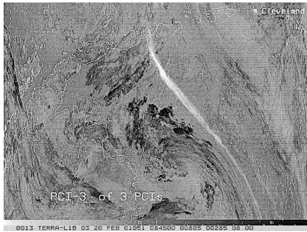
FIG. 12. PCI-3 of three PCIs that were generated from a simulation of the three thermal infrared bands of GOES-8 through -11 (bands 2, 4, and 5) using MODIS bands 22, 31, and 32 for 0845 UTC (nighttime) 20 Feb 2001 over Cleveland volcano in the Aleutian Islands. PCI-3 shows the ash cloud (white) by heavily utilizing GOES bands 4 and 5.
