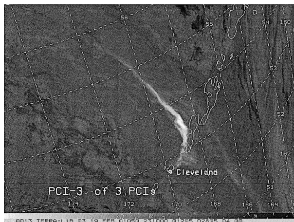
FIG. 9. PCI-3 of three PCIs that were generated from a simulation of the three thermal infrared bands of GOES-8 through -11 (bands 2, 4, and 5) using MODIS bands 22, 31, and 32 for 2310 UTC (daytime) 19 Feb 2001 over Cleveland volcano in the Aleutian Islands. PCI-3 shows the ash cloud (white) by heavily utilizing GOES bands 4 and 5.
