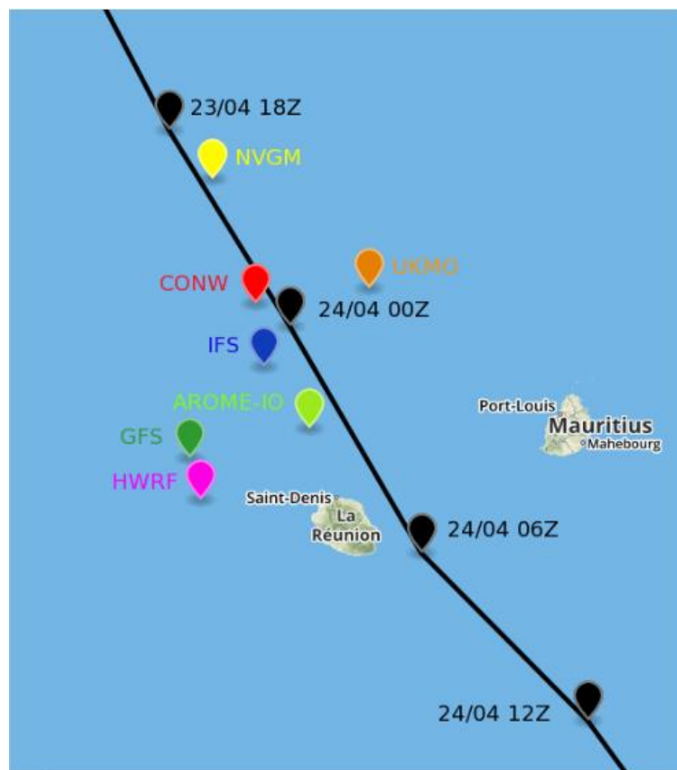
23/04 00Z run guidance forecast positions for the 24/04 06Z (H+30) (colored spots), Bestrack (black spot/line)
