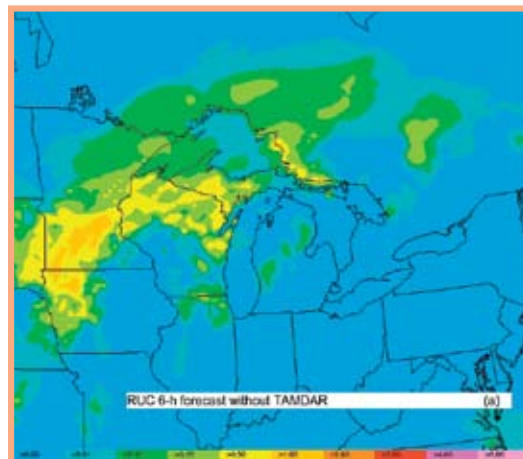
Fig. 7. RUC 6-h forecasts, ending 0600 UTC 5 October, of accumulated precipitation (in) (a) without TAMDAR; and (b) with TAMDAR.
