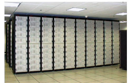
Figure 1: An illustration of Jet. The nearest "wall" contains one hundred processors with ten systems per column and ten columns. Each Compaq Alpha system is rack mounted in standard desktop system boxes.
