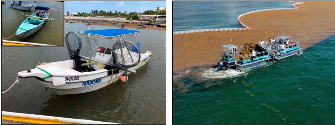
Figure 3-7. Examples of Sargassum collection devices. Left: The littoral collection module (LCM), a net system that can be fitted to a small vessel. It is deployed by rotating the net into the water. Source: Gray et al. (2021). Right: An example of a Sargassum harvesting system (Sargaboat). Sargassum is contained by a high boom that will not get overwhelmed by debris, and then collected using a vessel with a conveyor belt that skims Sargassum from the surface of the water and loads it onto a collection barge. Similar designs are based on aquatic weed harvesting vessels modified for use in marine waters. Source: https://theoceancleaner.fr/our-boats/
