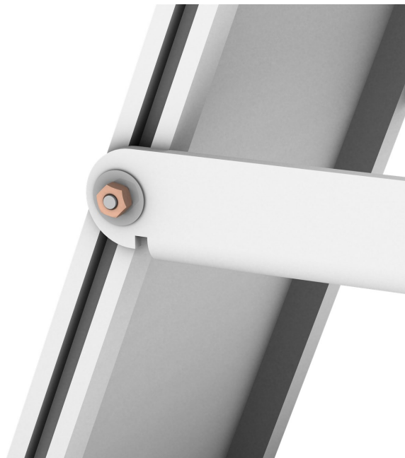
FIGURE 3-15. Adjust the tilt angle of the SP10
