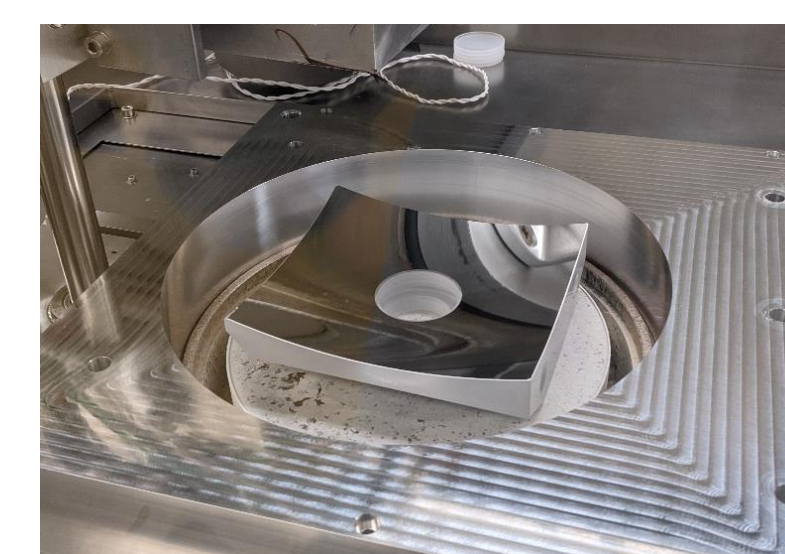
SPRITE CubeSat primary mirror 16 x 18 x 5 cm in the JPL ALD chamber
