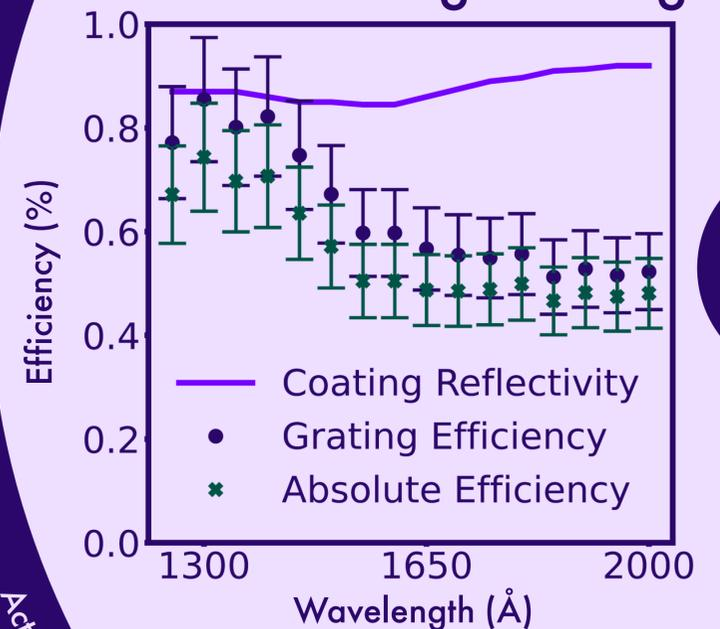
Xenon-enhanced lithium fluoride, an ultraviolet reflective coating developed at Goddard Space Flight Center, has been successfully applied to replica holographic gratings.
